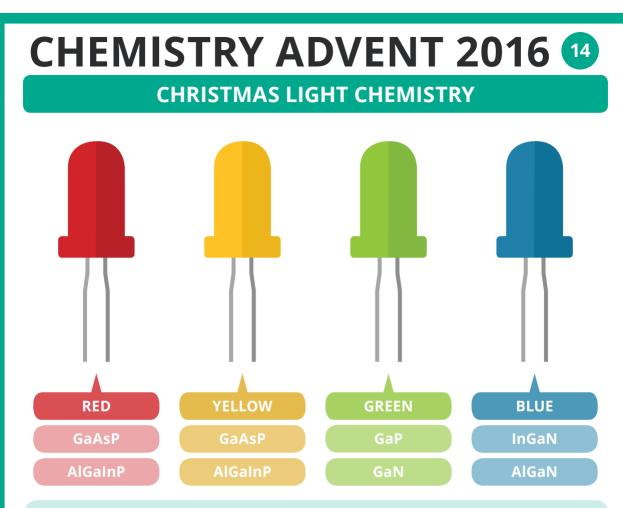
LEDs (light-emitting diodes) give off light when current is passed through them. They are made from semiconducting materials; the colour of light emitted depends on the materials used. Many of these materials are based on gallium, such as gallium arsenide phosphide (GaAsP), gallium phosphide (GaP), gallium nitride (GaN), and aluminium gallium indium phosphide (AlGaInP).
